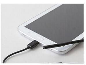
OTG adapter from micro USB to USB A, allows you to use the endoscope on your computer and Android smartphone.
